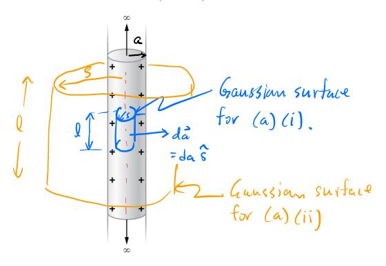
(b) Show that the electric fields calculated in (a) satisfy the boundary conditions for  $E_{\perp}$ . Assume that the pipe has thin walls and serves as the boundary separating the regions of space inside and outside of the pipe. (2 marks)
